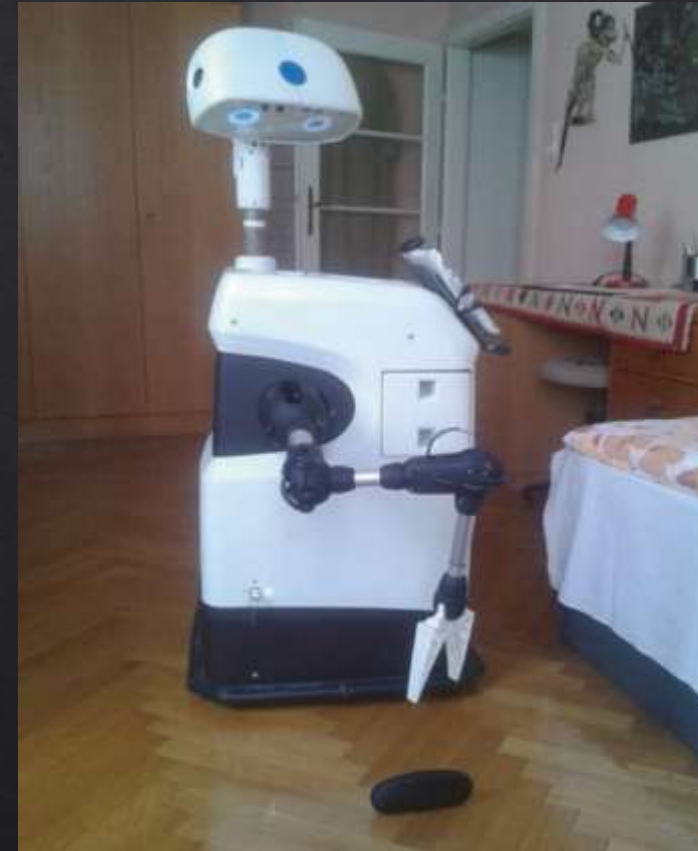
Hobbit – Bring-Roboter with fall-detection [PotentiAAL]
